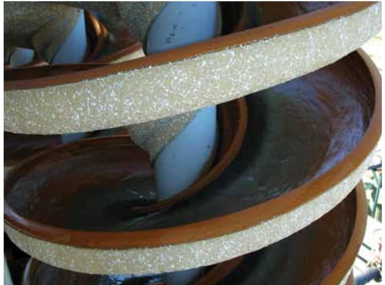
into distinct bands of materials of similar densities. Similar minerals are concentrated by splitters, which physically direct like bands of material onto the next processing step.
